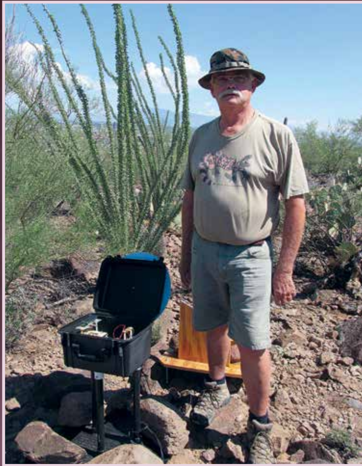
Carl Noggle stands beside his custom-built lightning sensors in Tucson. The sensors detect fast, high-current lightning as well as slow, low-current lightning. The latter has been known to start forest fires.
